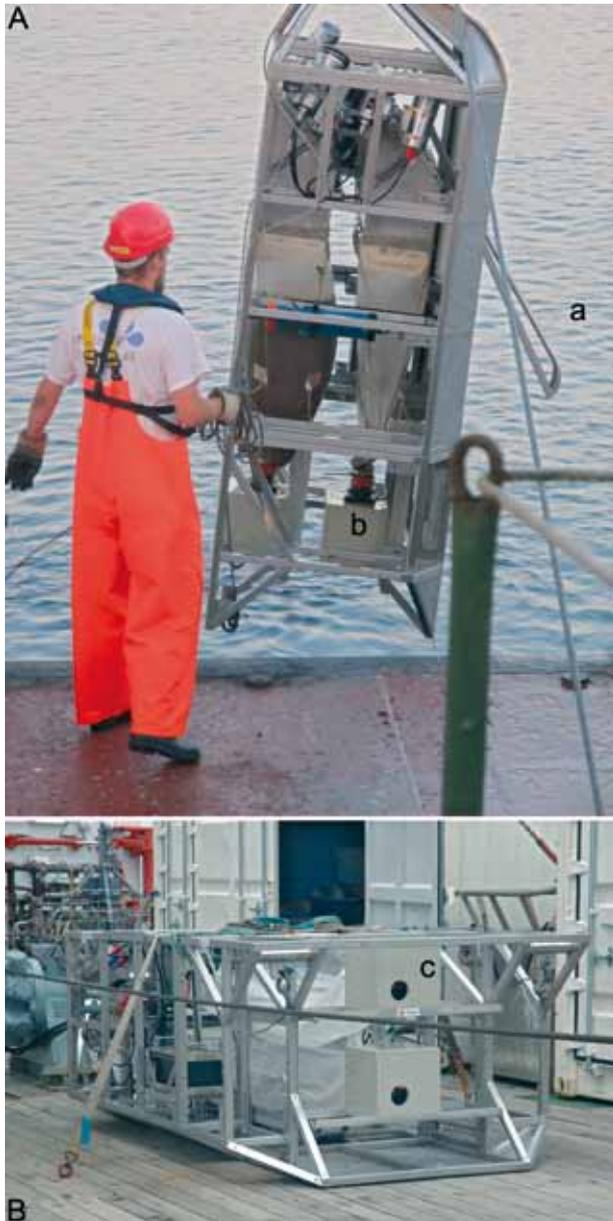
**Figure 1.** The thermo boxes on the Camera Epibenthic Sledge (C-EBS; Brandt *et al.* 2013) are able to reduce warming of the samples during retrieval through the water column. A.) While the C-EBS is veered and heaved through the water column, the lever is extended (a). The thermo boxes (b) are closed. B.) When the C-EBS is at the bottom, the lever is pushed in and the thermo boxes are thus open (c) to reduce dynamic pressure.
