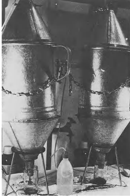
Fig. 12.2. Modified Berlese funnels used for soil extraction. The funnels were placed in a cool room (17°C)
